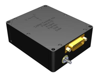
The Hi-Rel Magnetometer FGM-A-75 is an instrument for measuring three-dimensional magnetic fields. It is based on the fluxgate principle, using three independent ringcore sensor heads for each orthogonal axis. The technical performance data of the FGM-A-75 are based on an ESA qualified unit.
