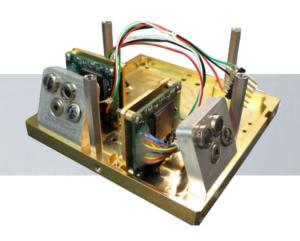
The MAI-SES is a miniature Static Earth Sensor suitable for CubeSats, NanoSats, and larger spacecraft in Low Earth Orbit.
