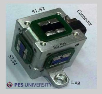
$4 \pi$  Sun Sensor is used in Spacecrafts to find the orientation with respect to Sun. Sun Sensor consists of two optical heads each head has solar cells mounted on three orthogonal sides. Two such heads mounted on two diametrically opposite side of a Satellite gives three direction cosines.
