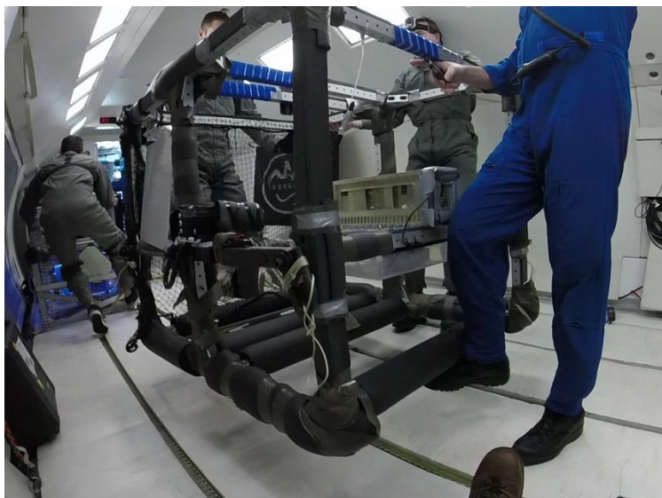
Figure 14-4: Test structure floating during micro-gravity test
