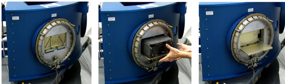
Figure 24-1: 6U payload deploying through ESPA port. CSD mounted directly via +Z face.
