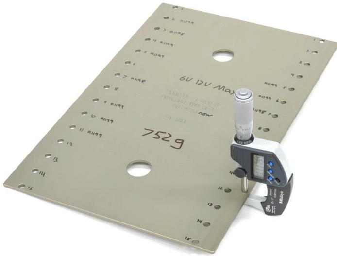
Figure 11-3: Measuring tab thickness with micrometer
