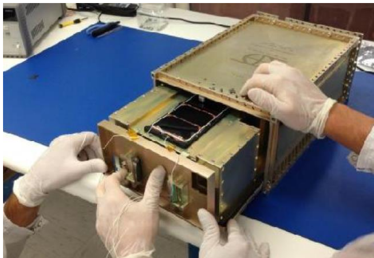
Figure 20-1: Installing 6U payload in CSD
