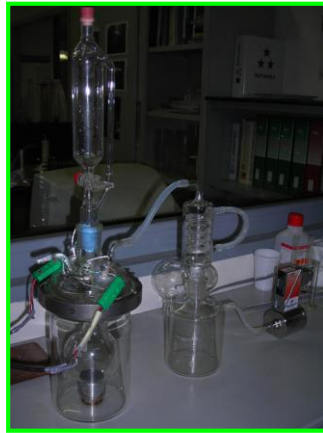
A schematic drawing (left) and a picture (mid) of SITAEL's test bench for the characterization of the catalysts. Picture of the main bottle of the test bench during the decomposition reaction (right)
