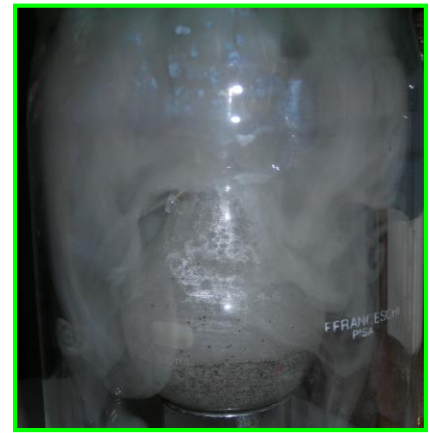
A schematic drawing (left) and a picture (mid) of SITAEL's test bench for the characterization of the catalysts. Picture of the main bottle of the test bench during the decomposition reaction (right)
