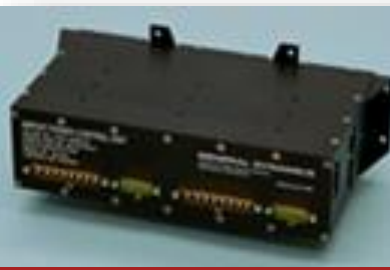
EO-1 High Voltage Power Conditioner
